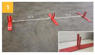
All Modu-Loc fence bases consist of one square and one round peg. Lay out fence bases 10 ft apart with all of the round pegs facing the direction you will build your fence.
